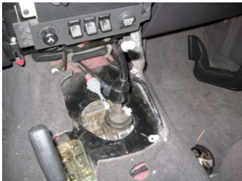
Manual Shifter (and trans plate with hole cutout in it)
