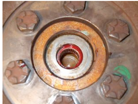
Pilot Bearing Installed
