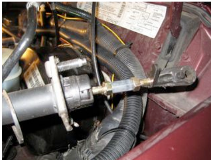
Cut & Extended master cylinder rod
