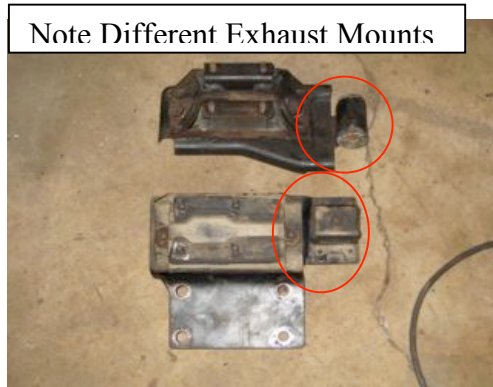
Different Trans mount brackets (Bottom one is for manual)
