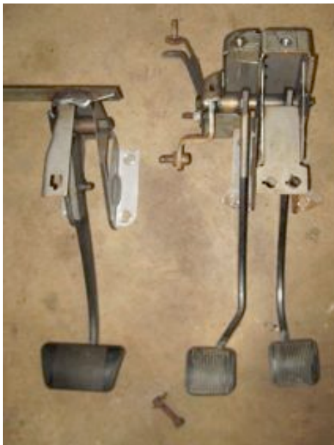
Clutch/brake pedal comparisons. Notice the difference in length of the brackets
