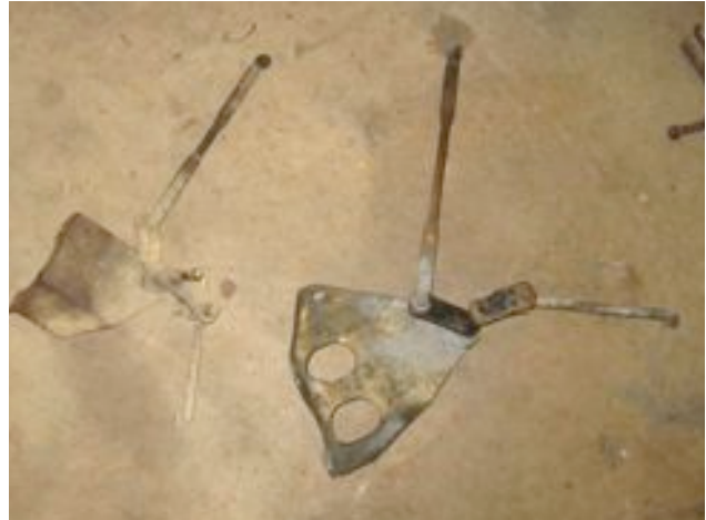
Different Linkage – Left=Manual Right=Auto
