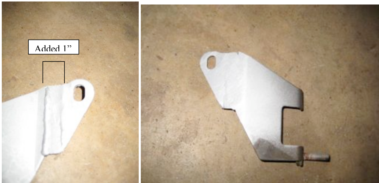
Clutch master cylinder brace with about 1" added
