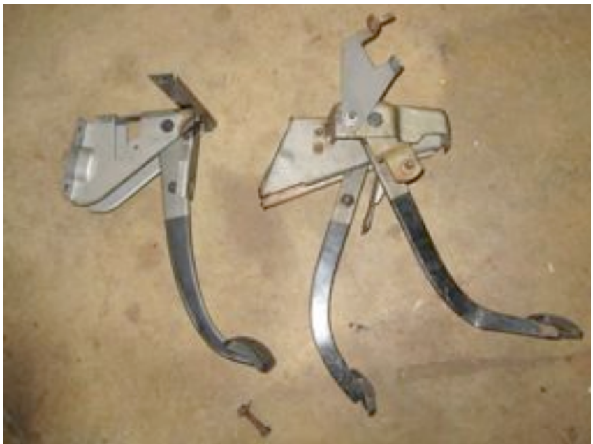
Clutch/brake pedal comparisons. Notice the difference in length of the brackets
