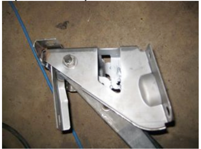
Removal of the clutch pedal part of the assembly.
