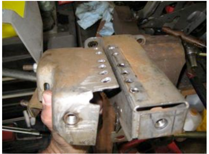
Removal of the clutch pedal part of the assembly.
