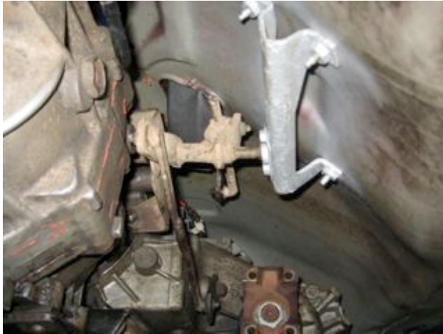
Shift Linkage Installed
