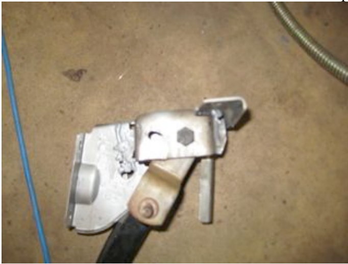
Removal of the clutch pedal part of the assembly.
