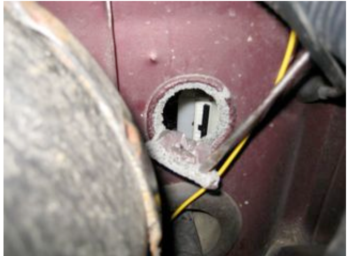
Plug just pops out with a screwdriver
