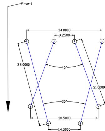
Note: All links are centered left to right, on both axle, and between frame rails.
